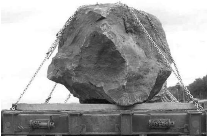
Chain is used to secure large boulders
